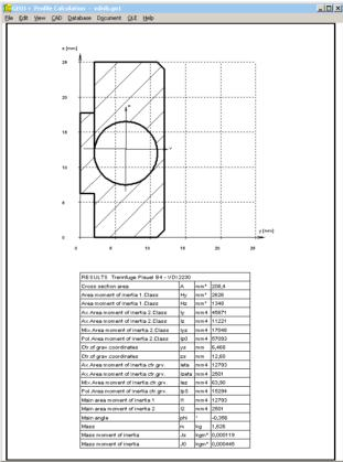
Calculated by means of GEO1+ with Ages=272mm<sup>2</sup>: IBT = 2822 mm<sup>4</sup>
