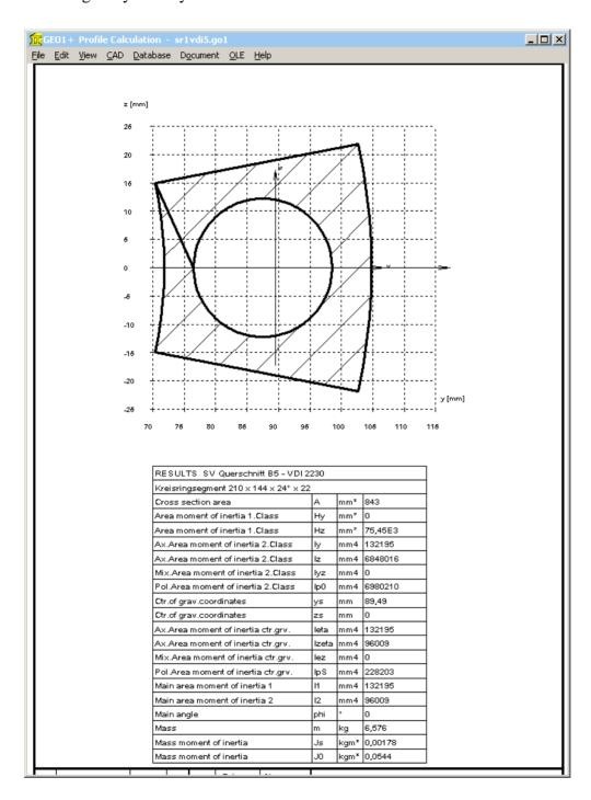
With coordinates of interface area are ri=72mm, re=105mm, alpha =  $24^{\circ}$ , rS=87.5mm and dh=22mm, GEO1+ calculates ys=89.48 mm. Thus ssym = ys – rS = 89.48-87.5 = 1.98 mm, u = ys – ri = 89.48-72=17.48 mm, and v = re - ys = 15.48 mm. Area moment of inertia at w axis is Izeta= IBT = 95985 mm<sup>4</sup>.
