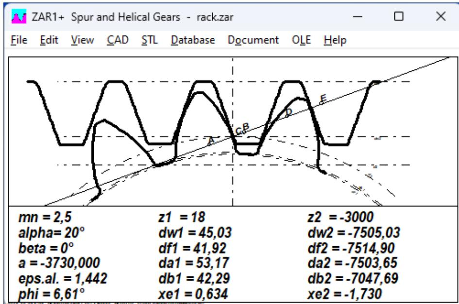
For the rack-pinion calculation, a rack is a gear with an infinite number of teeth. In ZAR1+, it is recommended to use a ring gear with 3000 teeth as the rack ( $z2 = -3000$ ).
