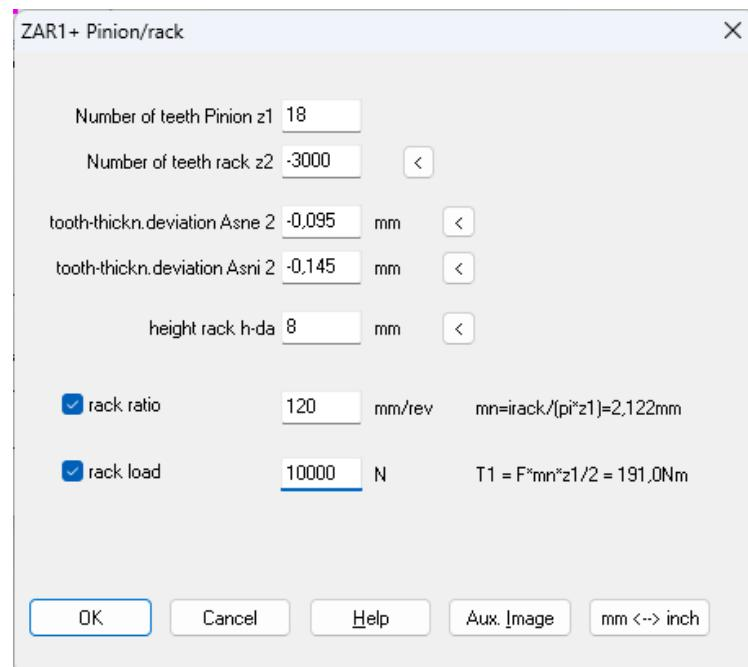
In the input window at "Edit\Special dimensions\pinion-rack" you can enter the tooth thickness tolerances and the height of the rack, known from earlier versions.
