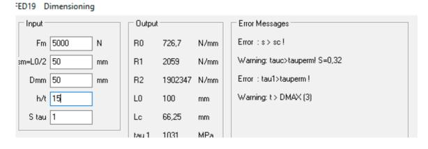
In the "recalculation" you can enter the dimensions of the spring (strip thickness, strip width, coil diameter at top/bottom, spring length, number of coils. For 2 spring lengths L1 and L2, FED19 calculates the spring forces F1 and F2.
