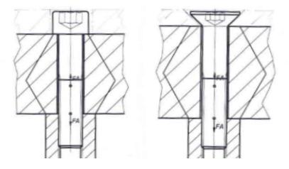
If a cylinder head screw is countersunk in the first clamping plate, the height of the first clamping plate must be reduced by the height of the screw head or the countersink, because the clamping plate is not clamped in the area of the countersink.
