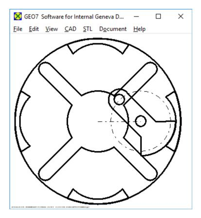
GEO7 calculates stepper gear with internal Geneva wheel. Interior Maltese have a long switching time and a short rest time compared to external Maltese gears. In a 4-beem external Geneva gear, the switching angle is 90 ° and the locking angle is 270 °. In case of an internal Geneva drive, the reverse is true: switching angle 270 ° and locking angle 90 °.
