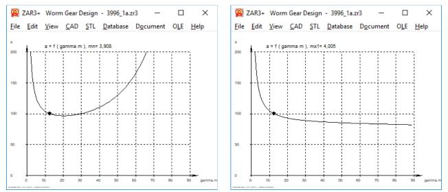
Diagram shows the smallest possible center distance, if mn remains constant. With worm gears, however, the axial modulus of the worm is normally specified, which corresponds to the tangential modulus of the worm wheel at 90 ° crossing angle (mx1 = mt2). Then mn = mt2 \* cos (beta2) and a0 = mx1 / 2 \* cos (beta2) \* (z1 / cos (summa-beta2) + z2 / cos (beta2))
