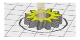
Up to now, only straight-toothed gears could be output as STL files for 3D printer production. This is now also possible for helical teeth. The helix is represented as a staircase function. Minimal stair width is the smallest possible layer thickness of the 3D printer. Suitable as an illustrative and functioning model, but rather unusable for practical use.
