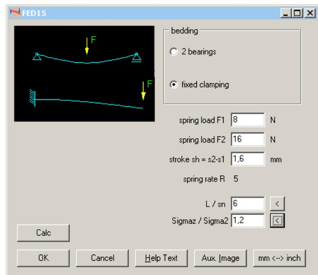
FED15 also provides a pre-calculation. Enter one or two loads and deflection, and FED15 calculates dimensions of the leaf spring. Modify ratio of spring length to deflection and safety sigmaz/sigma2 to vary leaf spring dimensions.
