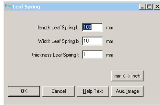
If the leaf spring geometry is just a piece of flat steel (as in FED15), you can now configure a simplified input for width, thickness and length of the leaf spring (at "Edit->Calculation method").
