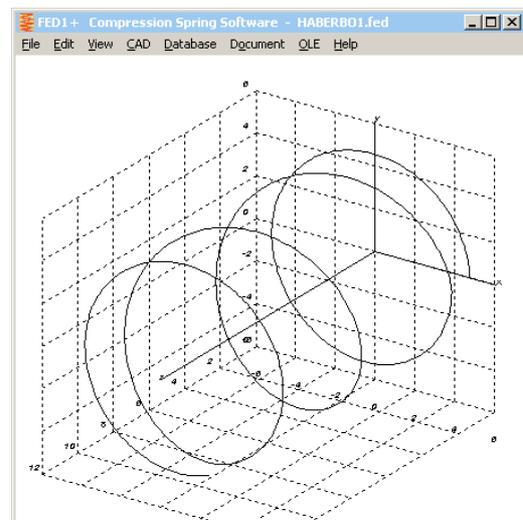
3D drawings are displayed on screen in a configurable xyz coordinate system, for DXF or IGES export, however, 3 dimensional with x,y,z coordinates. Now, you can configure at "File->Settings", if you want to export 3D drawings with xyz coordinates, or as 2D drawings in a coordinate system (same as the screen drawing). This option makes sense if 3D drawings are included in 2D drawings (production drawing, Quick3 view).
