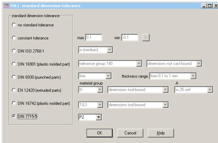
Tolerances according to DIN 7715 part 5 for elastomere parts has been added to the variety of selectable tolerances.
