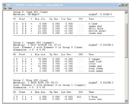
TOL2 is used in combination with our TOL1 software. First use TOL1 to define parts and components. In the next step, use TOL2 to assemble the TOL1 components by clicking TOL1 files and defining connection elements and connection tolerances.
