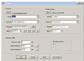
You can define several assembly conditions or switch positions and analyse the requested min/max values of the closing dimensions.
