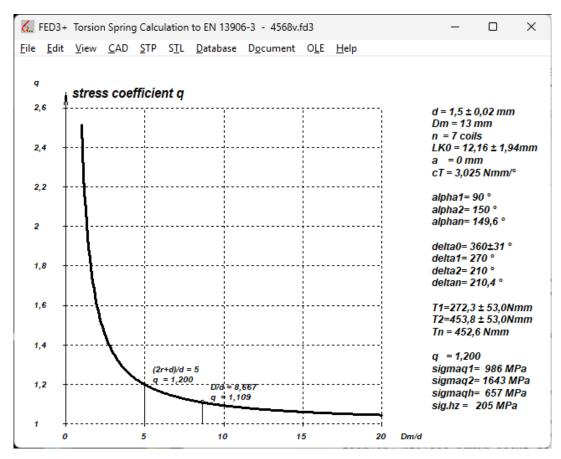
In FED3+ the diagram starts at w=1, in EN 13906-1 at w=2.5. The bending radius according to EN should therefore be at least as large as the wire diameter.
