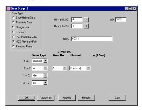
HCX planetary pair has, similar than Simpson or Ravigneux set, one or two input shafts, one output shaft and one idle shaft. Stepped planetary gears compared with simple planetary gears are used for larger transmission ratio.
