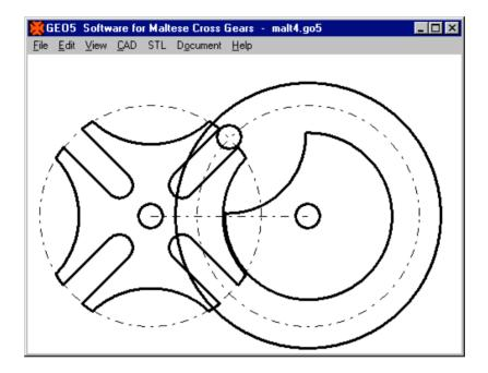
In an animation you can watch the motion of driving wheel and Maltese cross wheel on screen. Curves of travel, speed and acceleration are shown as diagram.
