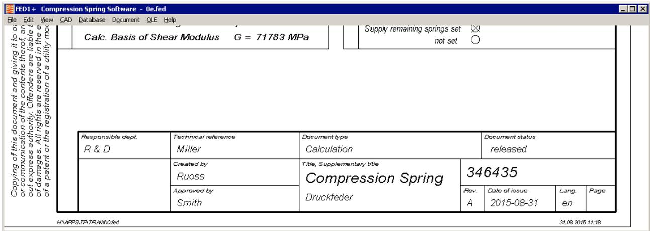
The drawing header of all production drawings and table drawings is configurable now (at "File->Settings->Drawing"). Default Setting is „ISO 7200 Fig.2“.
