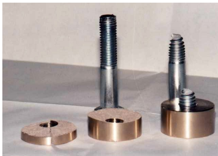
Fig. 3: Exploded bullet-panned shaped nut PAN 16 with screw M 20 x 110 from 5.6
