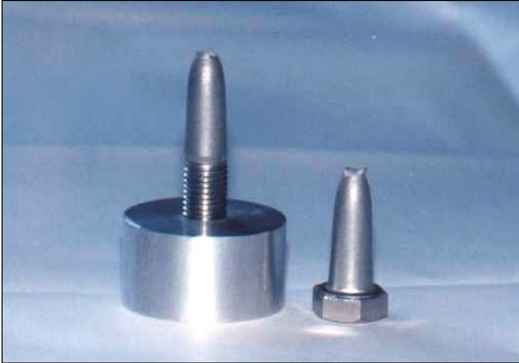
Fig. 4: Stainless Steel Screw A2-70, M 16 with Aluminum nut from 3.0615.71 (F 28) Length of thread engagement: m = 21 mm, Extension: 25 mm, Breaking load: F = 128 kN
